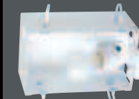
P4-TG Recessed Wall Box Size: 7-5/8" L., 4-7/8" W., 3-1/2" depth Lamp: 1 medium base, 75w max.
